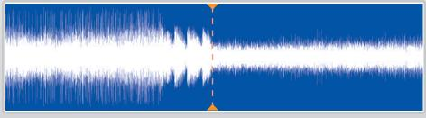
It is common in many scheduled maintenance programs to inadvertently overlubricate a bearing, and shorten its lifespan in the process. With ultrasound detection, it is possible to not only predict and verify when a bearing is needing greased, but also tell precisely when it is properly lubricated. Note the overlay on the sound file waveform above. This shows when the bearing has received exactly the right amount of lubrication.
